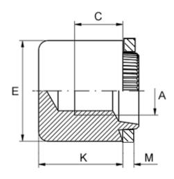
Female thread A = M3,5Height K = 9.0Min thread length C = 4.0Outer diameter E = 10.0Plate thickness = 4.7 to 4.9
